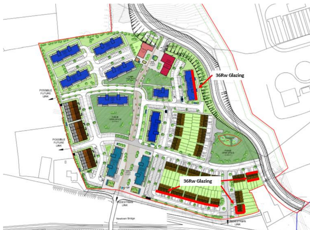
Figure 9.11 Enhanced Glazing Locations (Type A)
