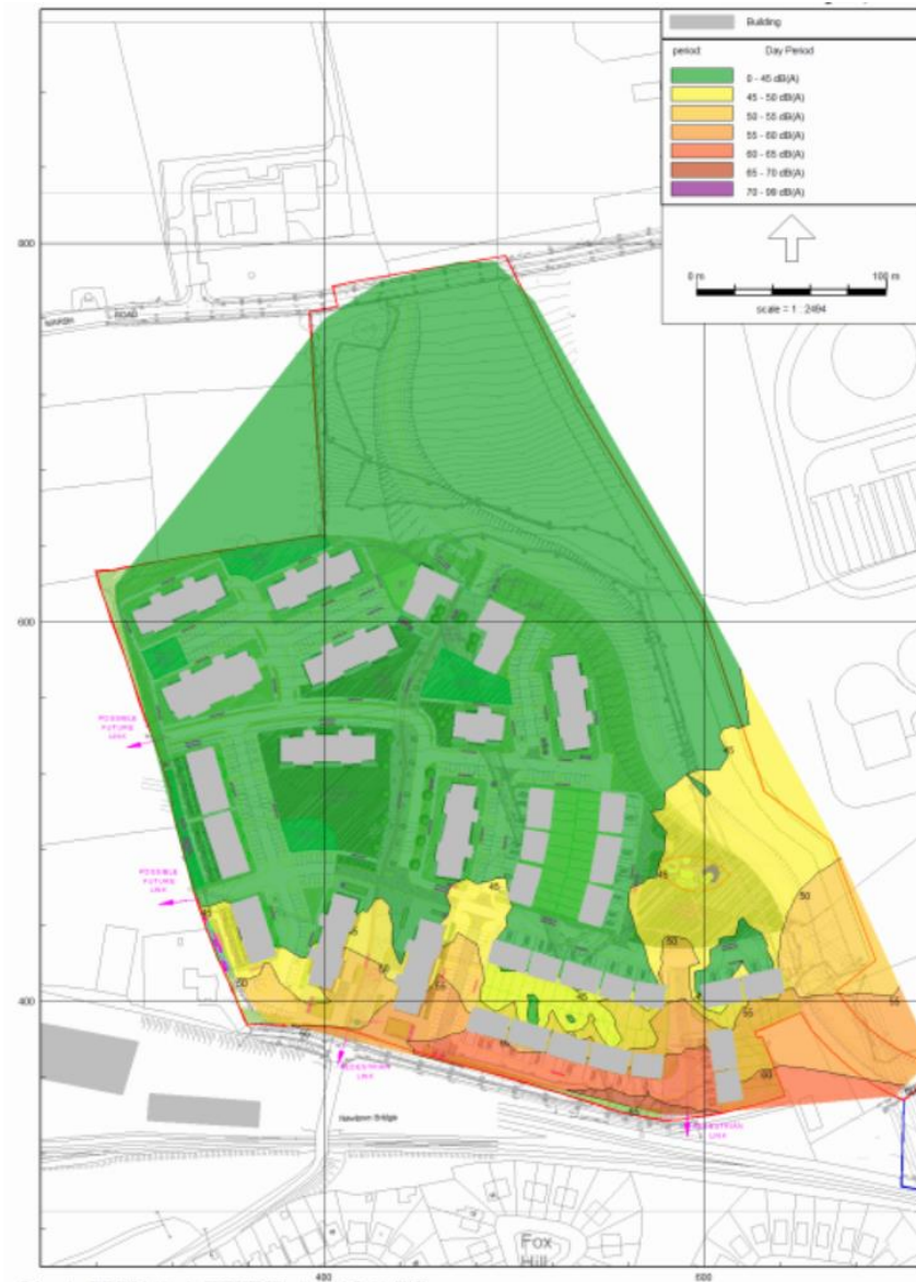
Figure 9.6 Rail Noise Levels with development buildings – Daytime
